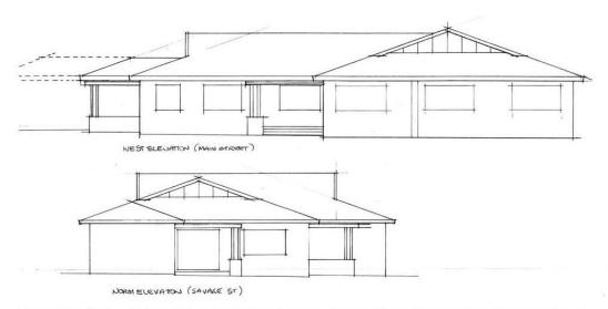
The major factor to take into account in changing the roof form from a flat skillion roof to a pitched roof is the differing structural conditions and upgraded structural standards. It is not simply a case of pulling one roof off and putting another on. We need to ensure the new roof structure is not only held up, but also held down.
